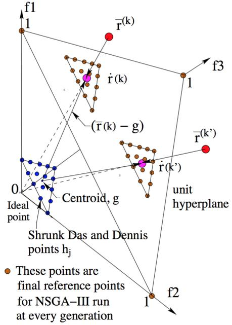
Fig. 1. A sketch of the R-NSGA-III's reference point  $\mathbf{Z}^a$  computation procedure.
